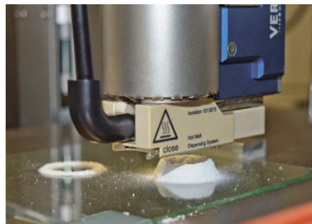
Heatable piezo valve dispenser (VERMES) printing thermoplastic
