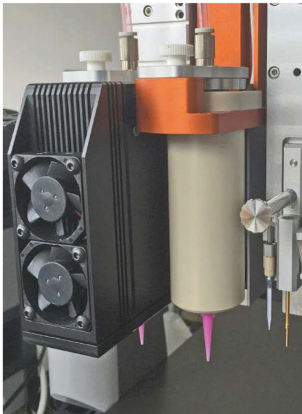
Peltier-cooled (left) and heatable cartridge holder, both actuated by compressed air. The right Z-axis holds a piezo pipette and a Z-sensor.
