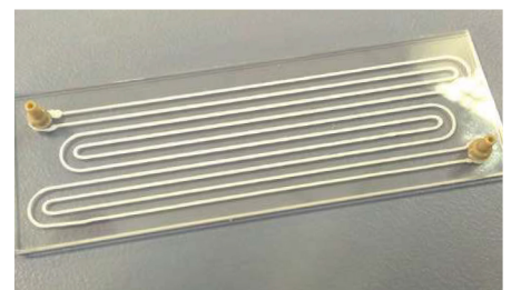
Top row: cylinders of polycaprolactone (PCL), MEW (100 PCL layers printed at 5 mm/s, 85 °C and 10 kV, no tear-off; strand thickness 15 \mu m) and a microfluidic channel printed on a slide. Bottom row: alginate scaffold and scanning electron micrograph of a bone cement scaffold after setting (material: InnoTERE, Radebeul).
