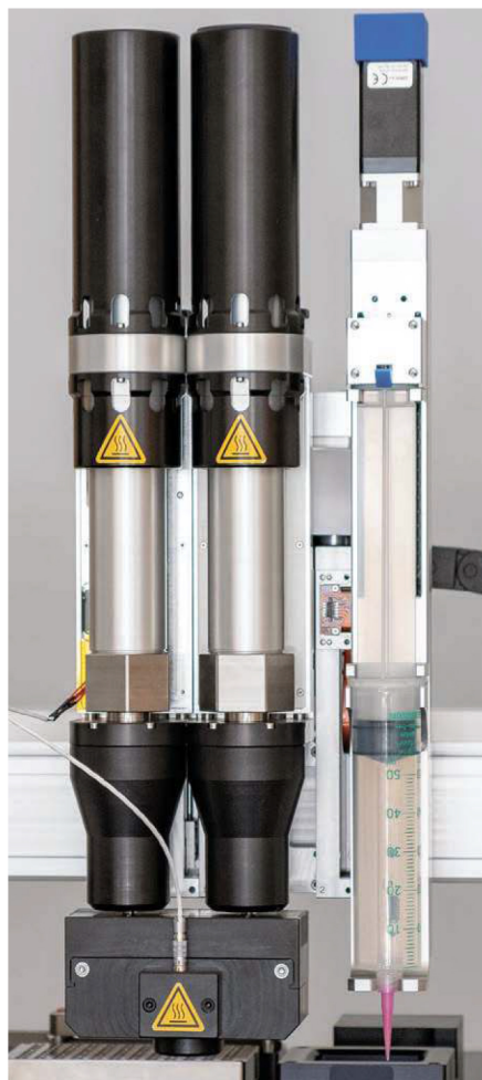
Mixing extruder (left) and piston extruder for 50 ml cartridges (right) in a BioScaffolder BS5.1. Note the two HT extruders on the gradient mixing chamber.
