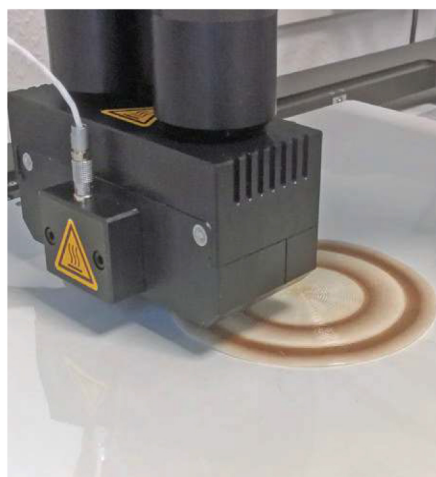
Concentric rings of coloured PEOT/PBT printed as a step gradient on a BS5.1
