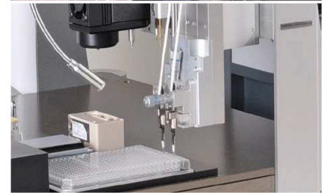
Twin-tip system with two piezo dispensers for in-flight/on target droplet mixing, with illumination (PTFE tubes not shown). Bottom picture: straight piezo dispensers for sample uptake.
